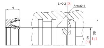
with PTFE materials, the profile size does not so much depend on the seal diameter but rather on pressure and extrusion gap. this relationship is described under "gap dimensions". nominal widths not shown in the diagram can be inter- polated.
