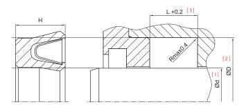
with PTFE materials, the profile size does not so much depend on the seal diameter but rather on pressure and extrusion gap. this relationship is described under "gap dimensions". nominal widths not shown in the diagram can be interpolated if required.
