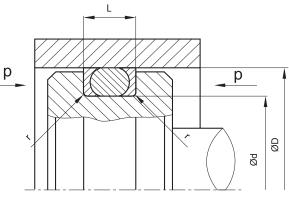
internal sealing (rod), back-up ring types, uncut & cut, r max 0,2mm
